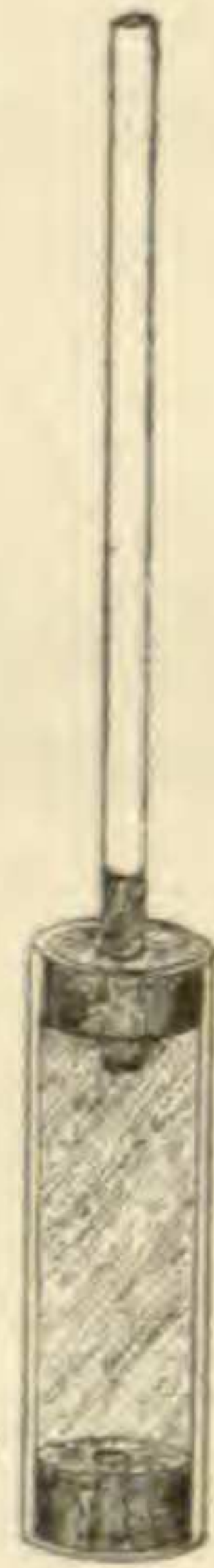
FIG. 3.—Osmotic apparatus used in testing directly the semipermeability of Xanthium seed coats; description in text.
